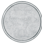
Erosion still permissible, plate can be polished
