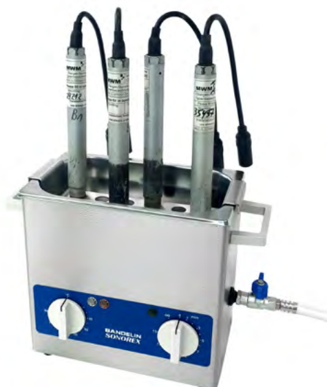
Ultrasonic bath SONOREX SUPER RK 102 H with spark plug holder
