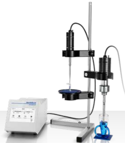
Sonication of two samples on one stand
