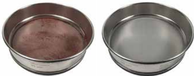
Test sieve before and after cleaning
