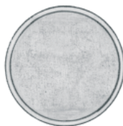
Erosion still permissible, plate can be polished
