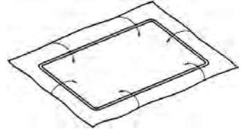
4. Place the covered foil test frame diagonally in the centre of the ultrasonic oscillating tank. Secure it if necessary.
