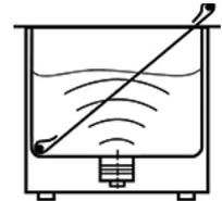
6. Switch off the ultrasound. Remove the foil test frame. Take the aluminium foil off the foil test frame and allow it to dry.
