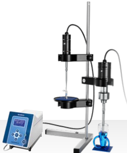
Sonication of two samples on one stand
