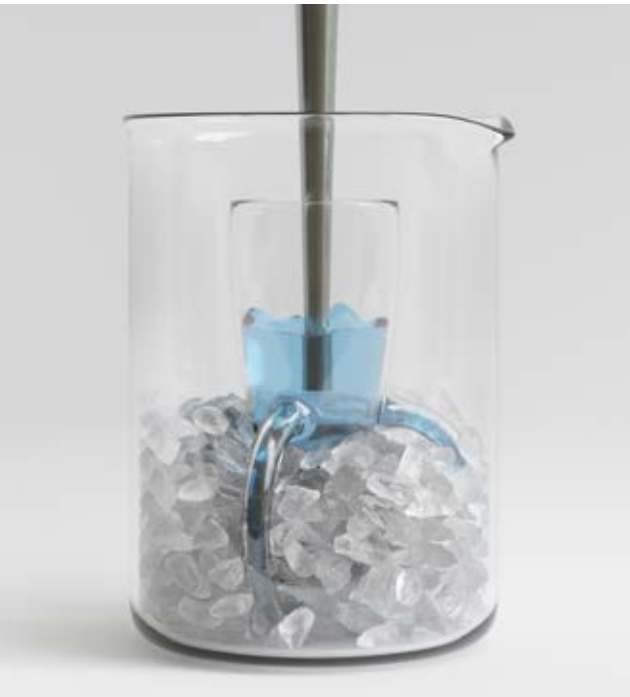
Cooling of the sample in a rosette cell RZ with crushed ice
