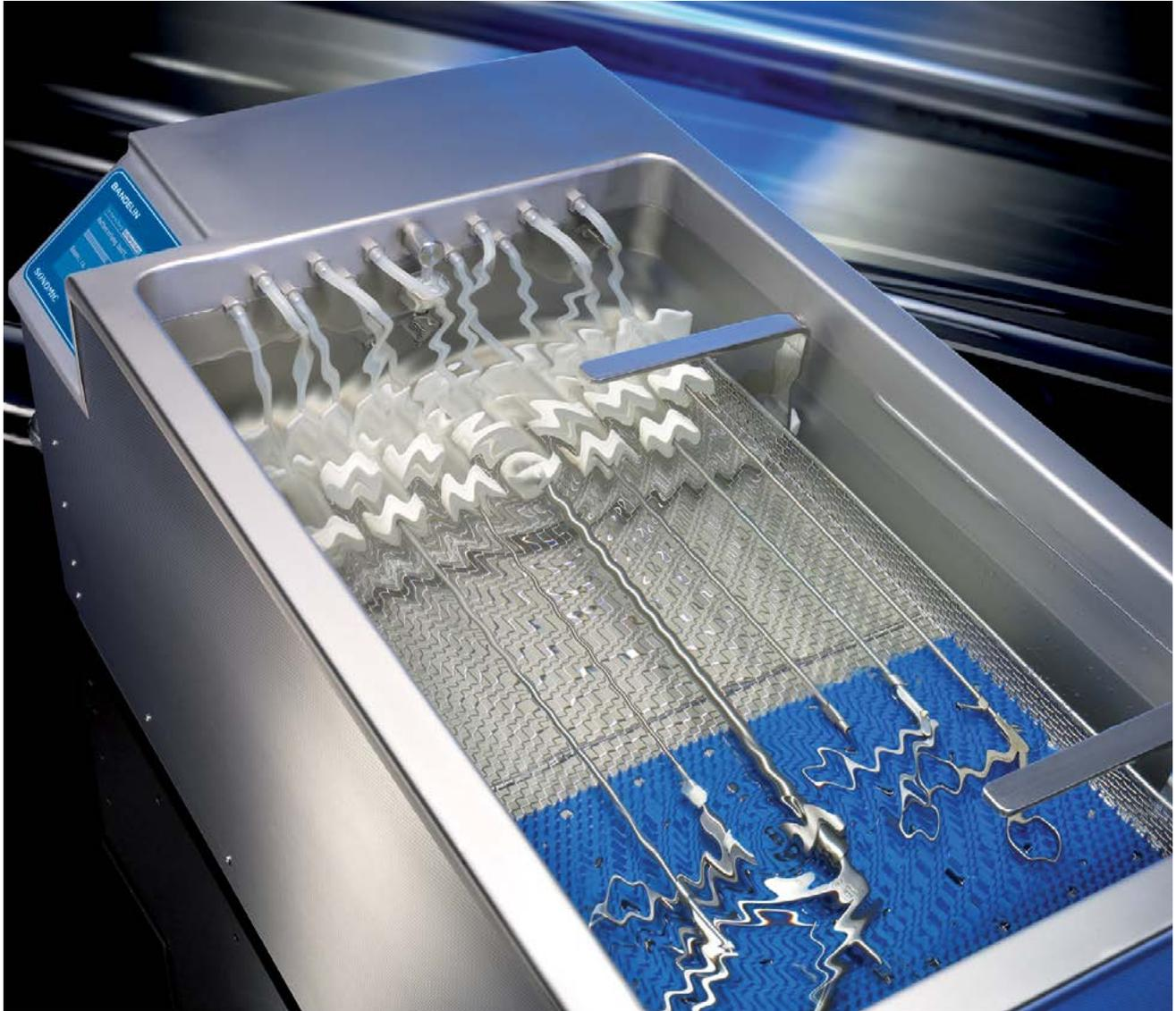
The reliable internal cleaning of MIS instruments and rinsable parts of other instruments ensures their continued use.
