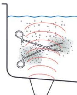
Foil after foil test in an ultrasonic bath with bottom sonication
