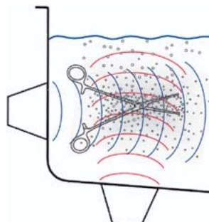
Foil after foil test in an ultrasonic bath with sonication from bottom and side
