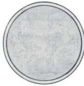
Erosion still permissible, plate can be polished
