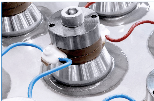
Close-up of an ultrasonic transducer
